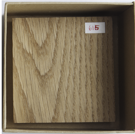
Figure 2: A material specimen as presented in its paperboard box (ash heartwood, specimen number 615)
