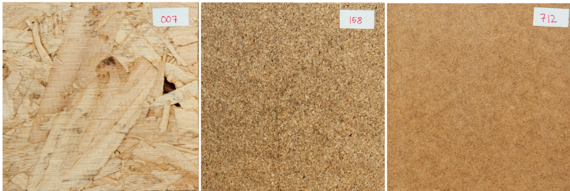
Figure 31: Three wood-based composites, each with greater degrees of transformation from their original state. From left: OSB, particleboard, MDF.
